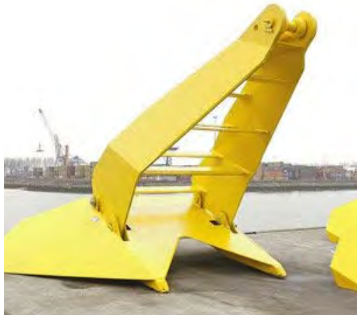
fig. 12 / Two piece drag embedment anchor
