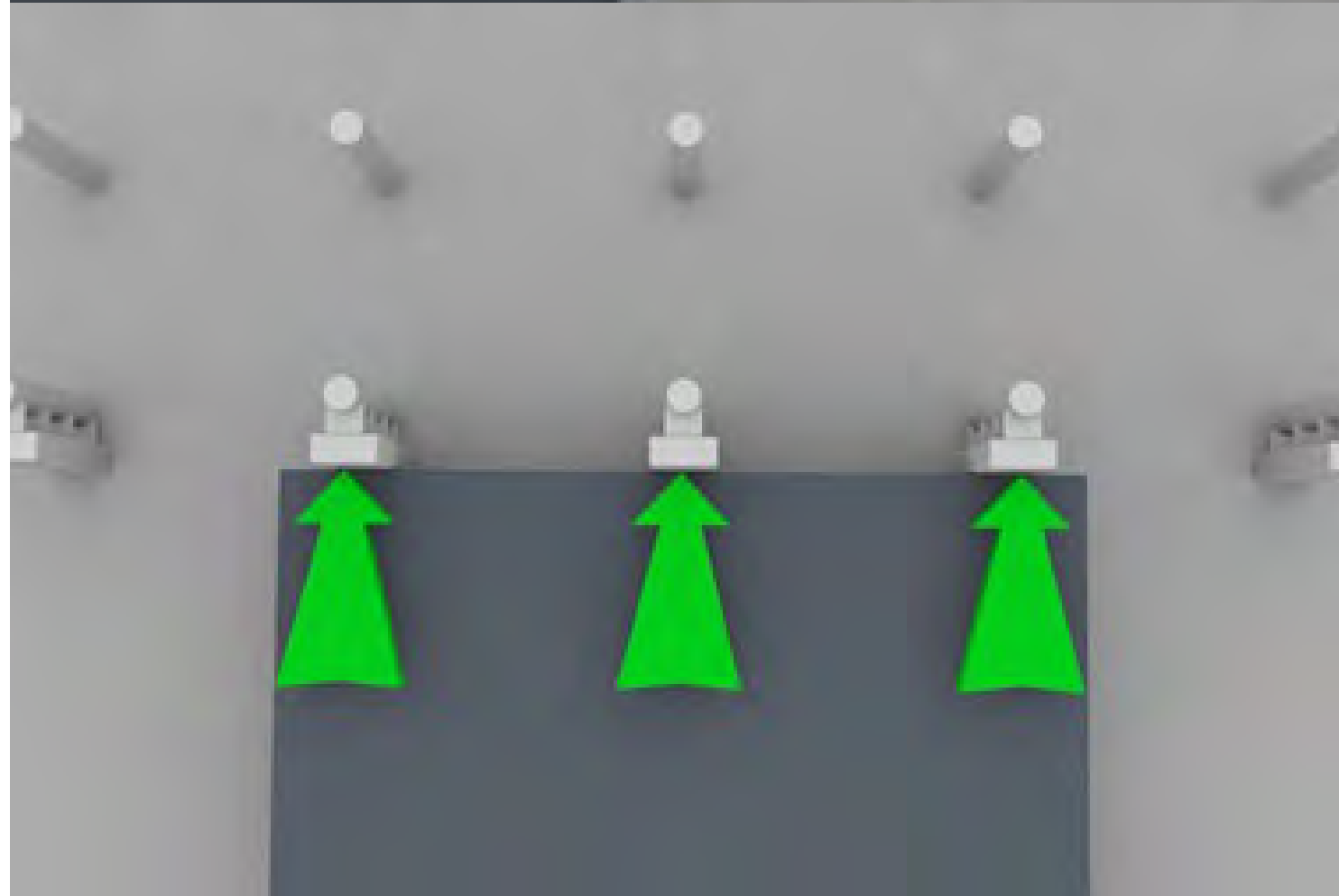
fig. 6 / Barge loadings on fendering at low water
